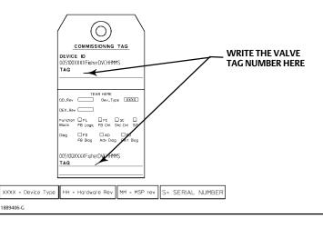
7. Remove the lower half of the paper commissioning tag and deliver it to the control system configurator. With the piece of paper, the control system configurator will be able to easily change the Device ID placeholder to the actual valve tag number.
