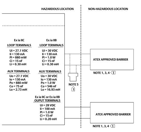
POWER MAY BE APPLIED TO EITHER THE LOOP TERMINALS OR OUTPUT TERMINALS OR TO BOTH SETS OF TERMINALS AT THE SAME TIME
