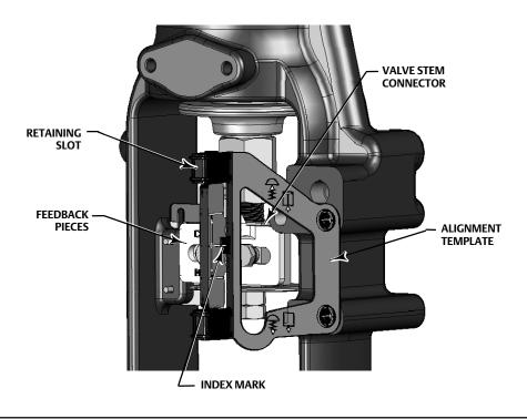
Figure 7. Air-to-Open Magnet Assembly Alignment
