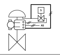
Figure 36. Tubing for Solenoid Valve Health Monitoring, Energize to Trip DVC6200 SIS
