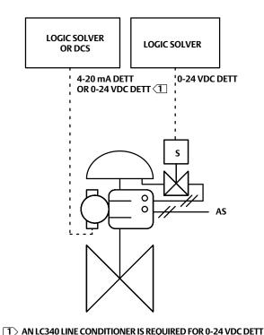
Figure 31. FIELDVUE DVC6200 SIS and Solenoid Valve Powered Together
