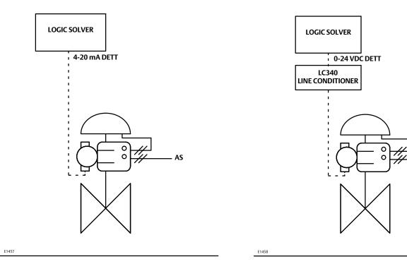
1. If the DVC6200 SIS is powered with 4-20 mA, connect the logic solver output card +/- terminals to the corresponding DVC6200 SIS LOOP +/terminals.
