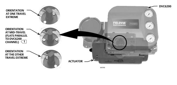
1 THIS EXAMPLE SHOWS AN ACTUATOR WITH 90° TRAVEL. ON AN ACTUATOR THAT HAS LESS THAN 90° TRAVEL THE MAGNET ASSEMBLY MAY NOT BE PARALLEL AT THE MID-TRAVEL POINT. TO VERIFY THE MAGNET ASSEMBLY POSITION IS IN WORKING RANGE, CONFIRM TRAVEL COUNTS ARE WITHIN THE EXPECTED RANGE OF 175-3800 USING VALVELINK SOFTWARE OR A FIELD COMMUNICATOR.
