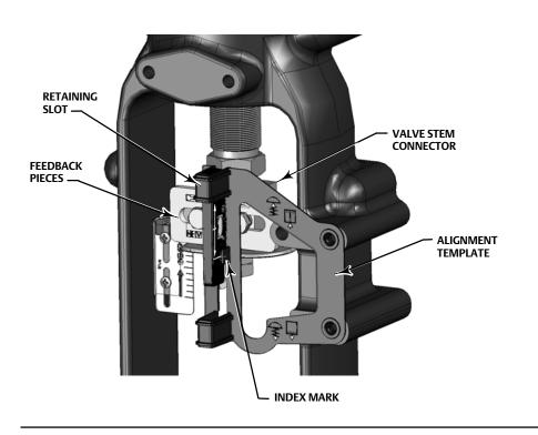
Figure 9. Air-to-Close Magnet Assembly Alignment
