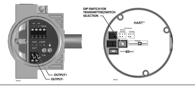
The position transmitter circuit derives its operating power from the control system input channel in the same manner as a 2-wire transmitter. The position transmitter circuit operates independently from the digital valve controller.
