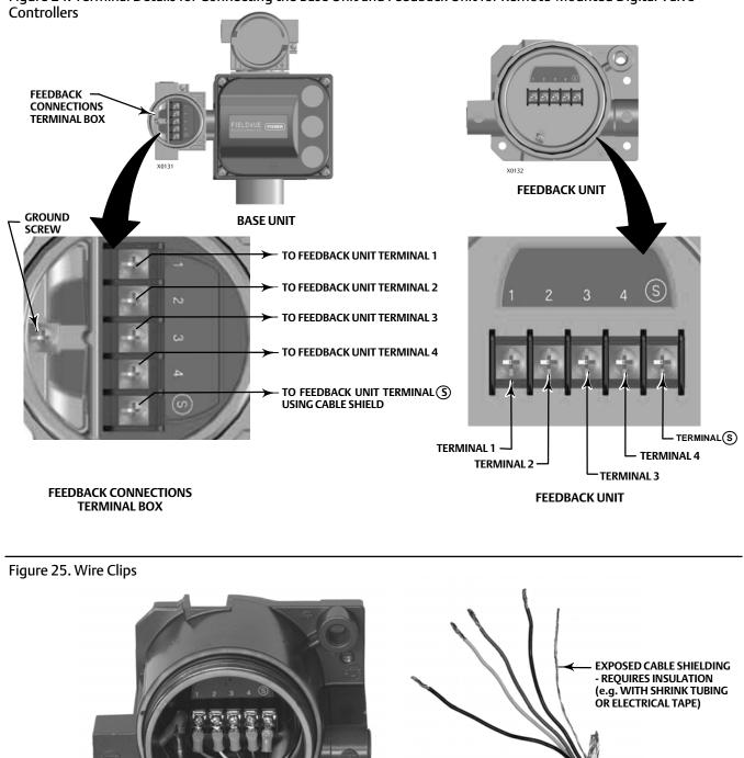
Figure 24. Terminal Details for Connecting the Base Unit and Feedback Unit for Remote-Mounted Digital Valve
