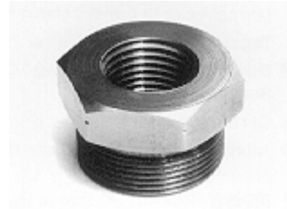
THERMOWELL ADAPTER KIT Adapting 1/2" MNPT Bimetal to 1-1/4"-18 threads for Industrial glass Thermometer Thermowell
