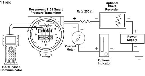
NOTE Signal Loop may be grounded at any point or left ungrounded. NOTE A HART Interface may be connected at any termination point in the loop. Signal loop must have 250 ohms minimum load for communications.
