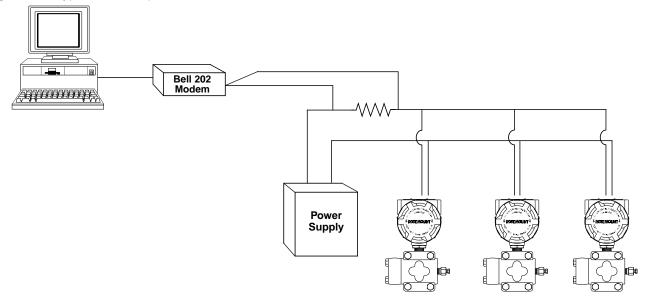
HART-based communicators can test, configure, and format a multidropped Rosemount 1151 in the same way as it can a Rosemount 1151 in a standard point-to-point installation.
