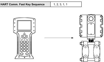
Reranging with only the communicator changes the analog 4 and 20 mA points independently without a pressure input.
