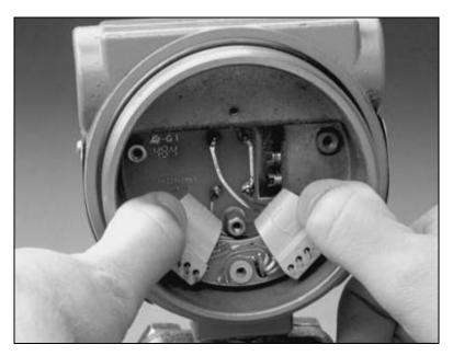
4. Align the smart electronics assembly with the bayonet connector pins, making sure all pins line up with the proper receptacles. Next, push the assembly slowly inward until it is fully seated.
