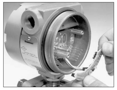
6. If the transmitter has linear output electronics, remove the three standoffs (4). Use a <sup>1</sup>/<sub>4</sub>-in. nut driver or wrench.
