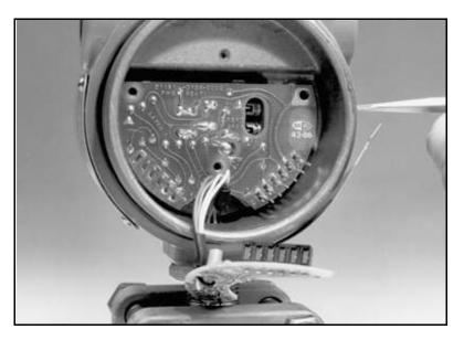
8. For linear output models, grip the calibration board (5) by the interface pin. (Removing the calibration board disables the conventional zero and span screws.)
