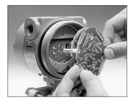
5. Pull the header board assembly (3) off the bayonet connectors. The header board must be reinserted. Do not cut the wires (9) or remove the header board.
