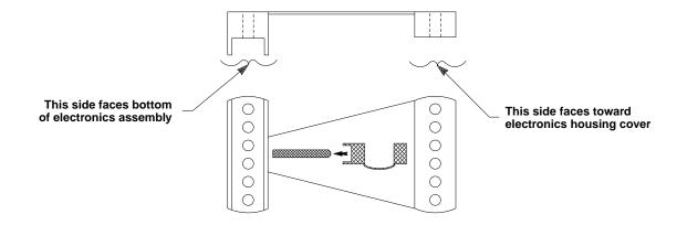
1. Slide the bottom half of one spacer over one of the rows of bayonet connectors. Then repeat the procedure for the other row.
