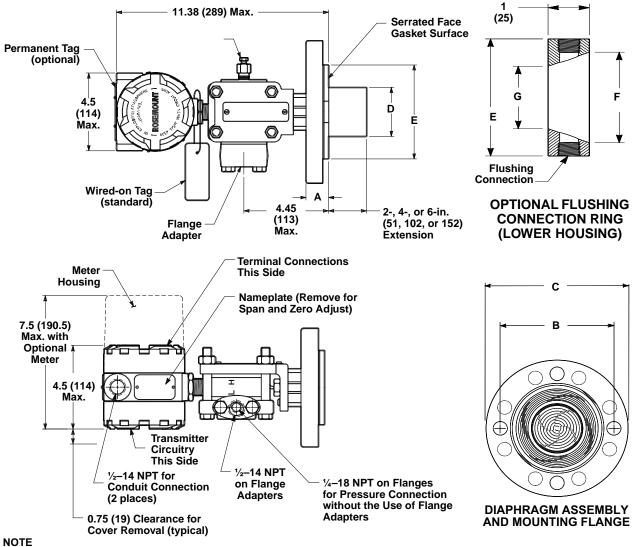
Figure 2-3. Rosemount 1151LT Dimensional Drawing.
