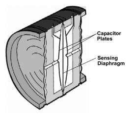
Second, transmitter span is also affected by static pressure. To understand this effect, it is necessary to understand the inner workings of the  $\delta$ -cell sensor.
