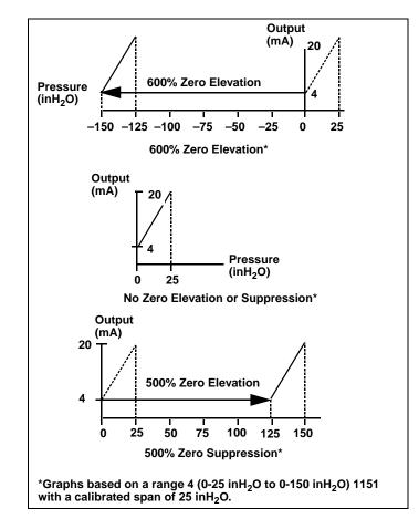
The zero may be elevated or suppressed to these extremes with the limitation that no pressure within the calibrated range exceeds the full-range pressure limit. For example, a Range 4 transmitter cannot be calibrated for 100 to 200 inH<sub>2</sub>O (24.8 to 49.7 kPa) (only 100% zero suppression) because 200 inH<sub>2</sub>O exceeds the 150 inH<sub>2</sub>O full-range pressure limit of a Range 4.
