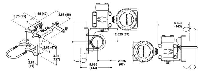
Figure 2-6. Mounting Bracket Option Codes B1, B4, and B7.
