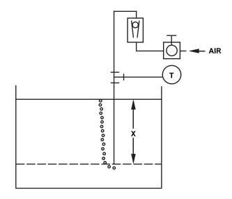
Let  ${\bf X}$  equal the vertical distance between the minimum and maximum measurable levels (100 in.).
