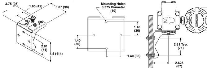
Figure 2-8. Flat Mounting Bracket Option Codes B3, B6, and B9
