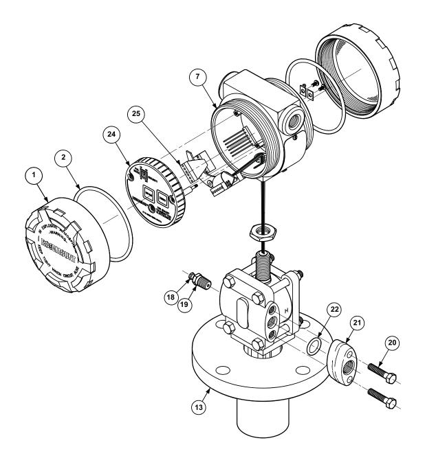
Figure A-5. Rosemount 1151LT Analog Pressure Transmitter Exploded View.
