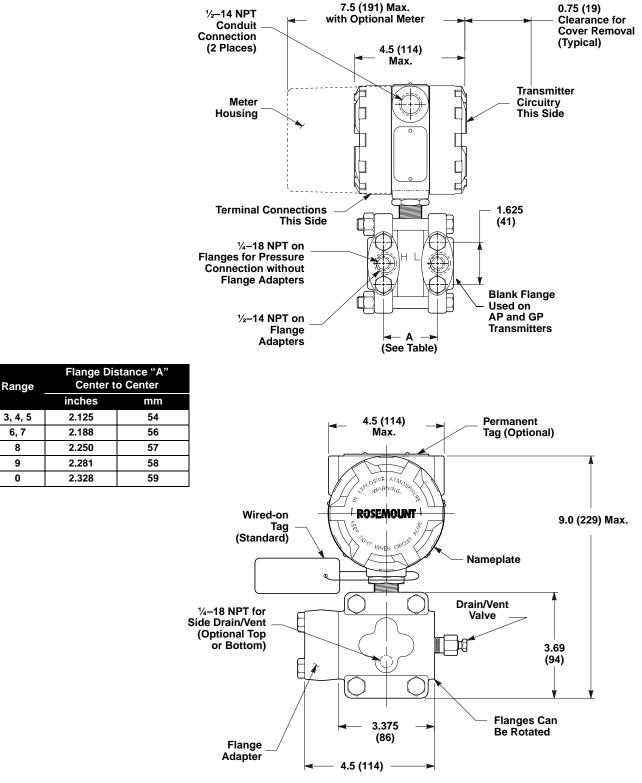
NOTE Dimensions are in inches (millimeters).
