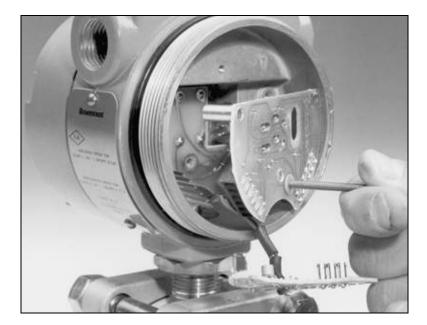
Insert the standoffs (7), if necessary. The transmitter is now ready to receive the plug-in smart electronics assembly.
