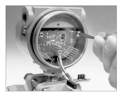
7. Align the zero and span adjust screws (10) so that the potentiometer blades are perpendicular to the board.
