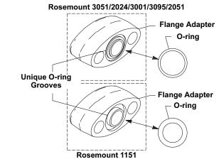
$\underline{\land}$  When compressed, PTFE O-rings tend to "cold flow," which aids in their sealing capabilities.
