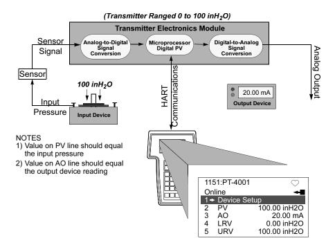
Figure 4-1 illustrates the Rosemount 1151 Smart transmitter data flow. This data flow can be summarized in four major steps:
