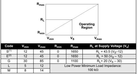
(1) A minimum of 250 ohms is required for communication.
