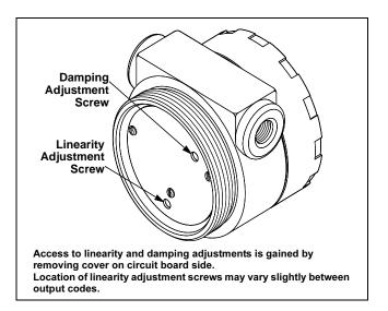
The amplifier boards for output options E and G are designed to permit damping of rapid pulsations in the pressure source through adjustment of the damping screw shown in Figure 4-11 on page -17. The adjustment is marked DAMP on the solder side of the amplifier board.
