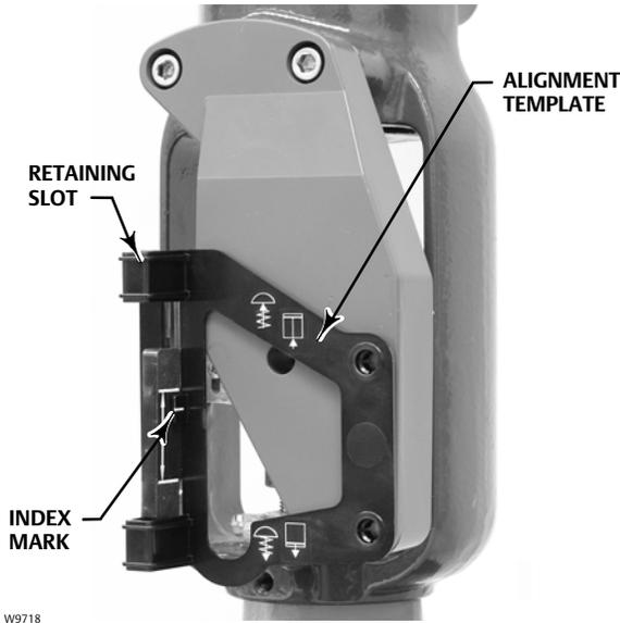
Figure 4. Air-to-Close Magnet Assembly Alignment
