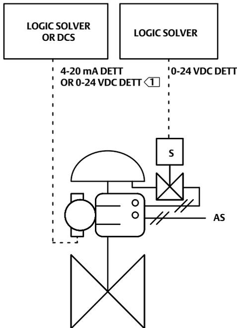
**1** AN LC340 LINE CONDITIONER IS REQUIRED FOR 0-24 VDC DETT
