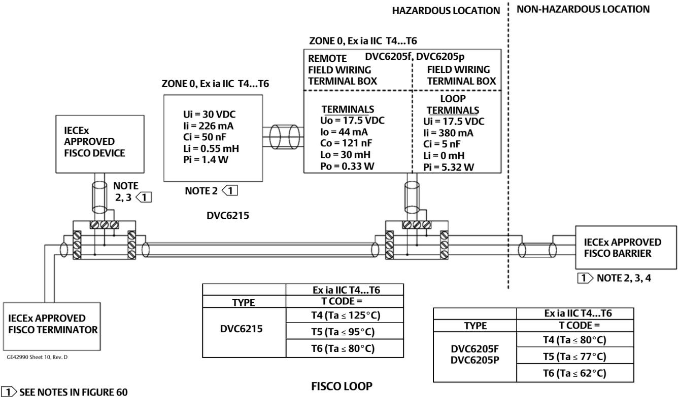
Figure 59. IECEx Schematic—FIELDVUE DVC6200 HW1
