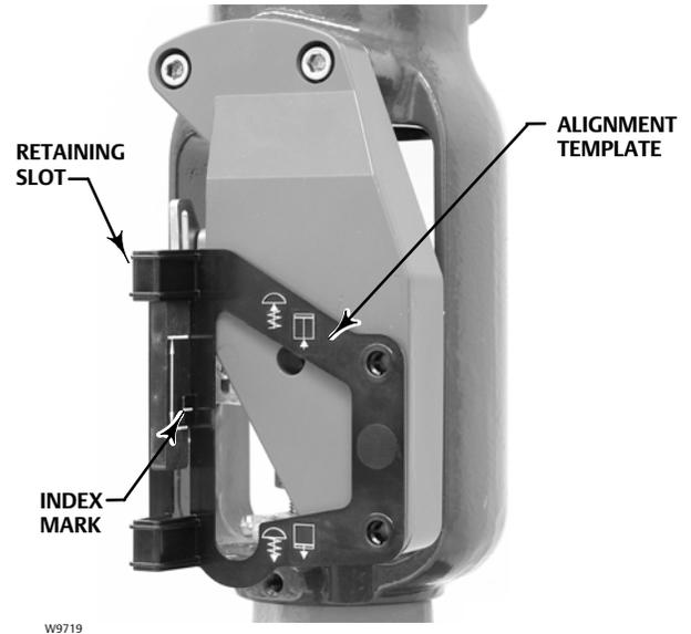
6. Tighten the fasteners and remove the alignment template.
