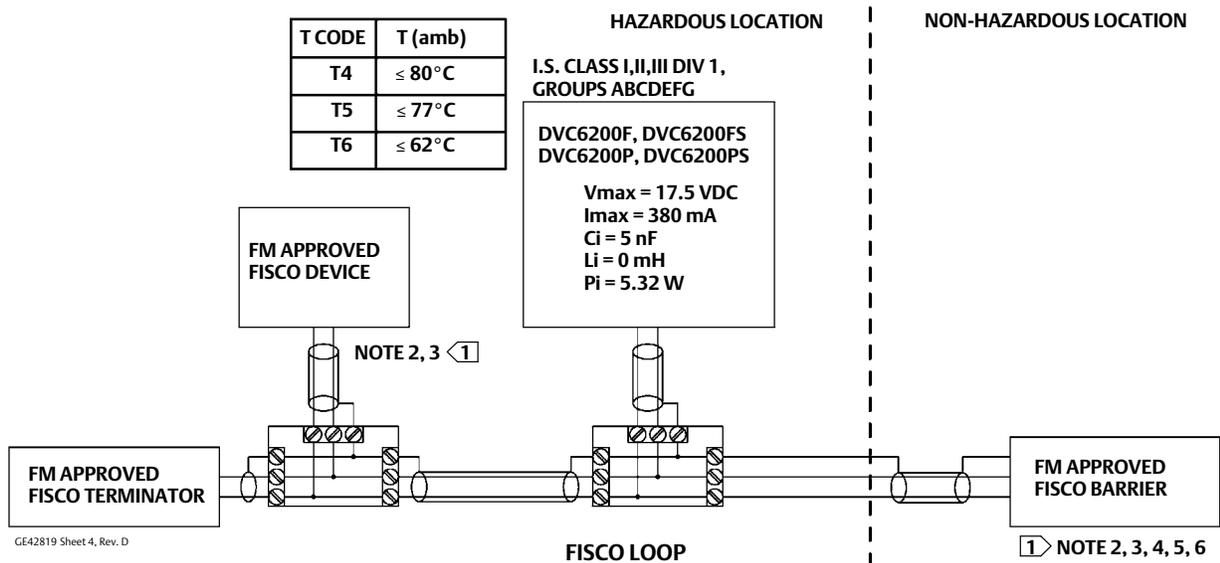
Figure 46. FM Loop Schematics—FIELDVUE DVC6205f, DVC6205p, and DVC6215
