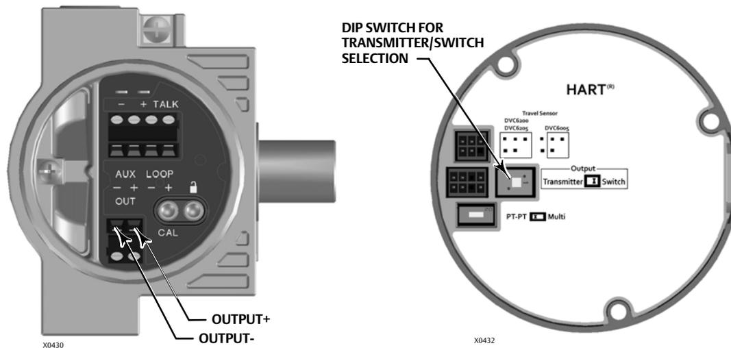
The position transmitter circuit derives its operating power from the control system input channel in the same manner as a 2-wire transmitter. The position transmitter circuit operates independently from the digital valve controller.
