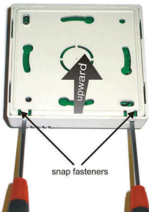
Fig. 14.1. Removal of the back wall
